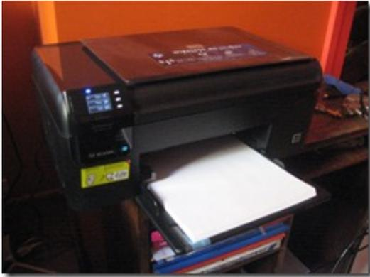
[1] I am reviewing the Hewlett-Packard B109n Photosmart Wireless[2]network multifunction printer which is HP's latest entry in to the basic network-enabled consumer multifunction printer market. It is based on their basic HP Photosmart printer, but has 802.11g WPA2 WPS wireless networking added to it.
